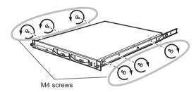
5 Insert the tags of the slide rail to the second hole from the bottom of the server.
